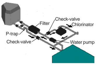
The pressure-type chlorinator or brominator takes a small amount of water from the outlet side of the filter, adds chemicals to it and returns this highly concentrated solution to the pool. The check valves must be highly resistant to corrosion. Use only a check-valve either supplied or recommended by the chlorinator (brominator) manufacturer.
